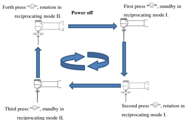
When the motor is in quick start mode, you can long press “P” to change the reciprocating speed and direction.
